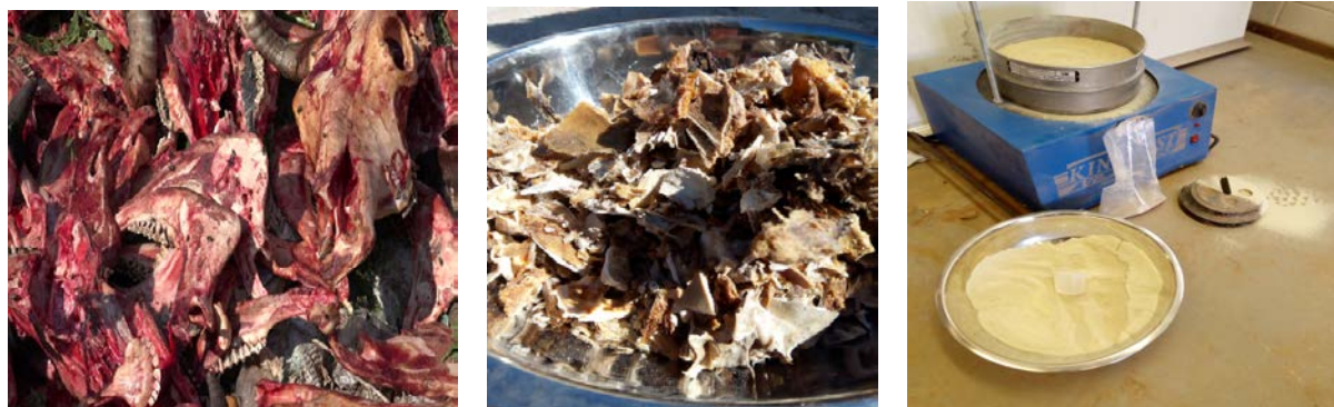
Figure 1: (a) Fresh Cow Skull Bone Obtained (b) Dried Cow Bone (c) Cow Bone Powder (CBP) in a 150 µm ASTM standard Sieve
