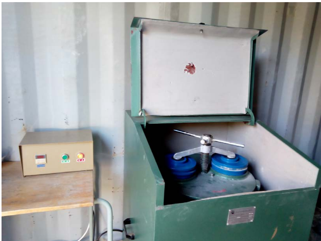
Figure 3: Diagram of Vibratory Disc Milling Machine (VDMM)
