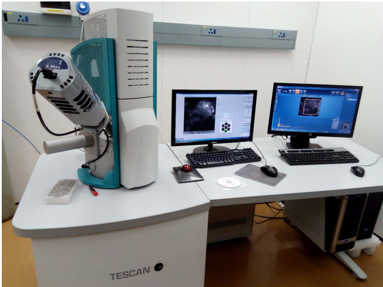
Figure 4: Photograph of the SEM-EDX Analysis Machine used
