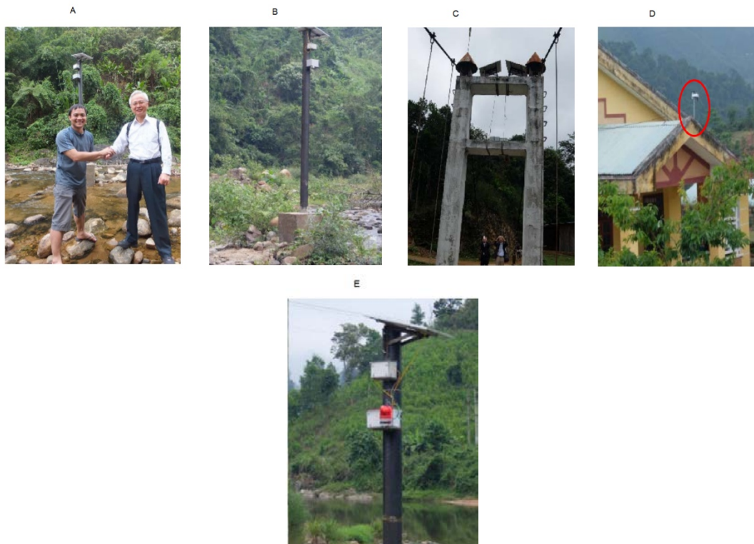
Figure 4: M2M direct interconnected devices installed in Namtramy district, province of Quang Nam, Vietnam (A and B: Sensors, C: Transmitter, D: Weather Station, and E: Connected Alarm for EWS)
