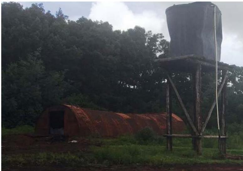
Figure 4: Metal kiln for carbonisation at Wattle Company Mimosa.
