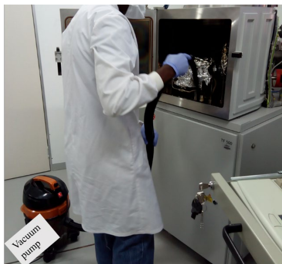
Figure 7. Vacuum cleaning of HHV TF500 system after a sputtering cycle
