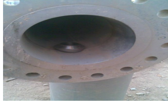
Figure 2. A real case illustrates missing sockolet
