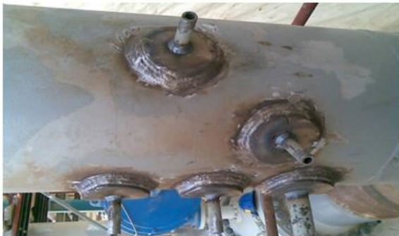
Figure 1. A real case illustrates missing spacer
