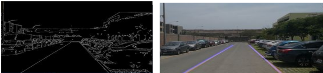
Fig. 3: Processing of images using algorithms that detect lanes
