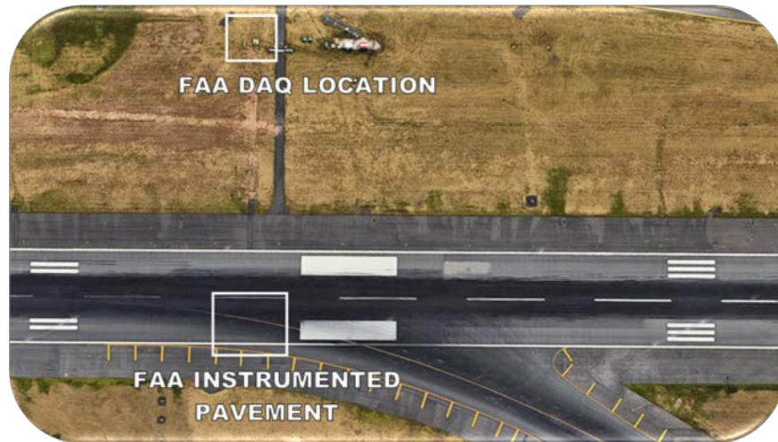
Figure 8. Location of instrumentation on runway (Imagery © 2016 Google, Map data ©2016 Google)
