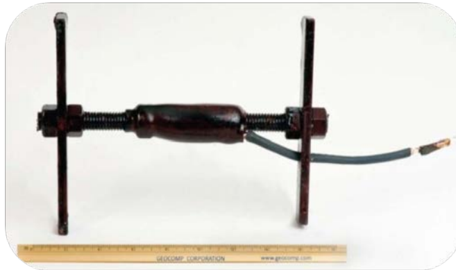
Figure 1. Typical strain gage for pavements
