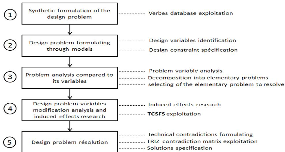
Figure 4. Proposed methodology to resolve induced effects problems in preliminary design
