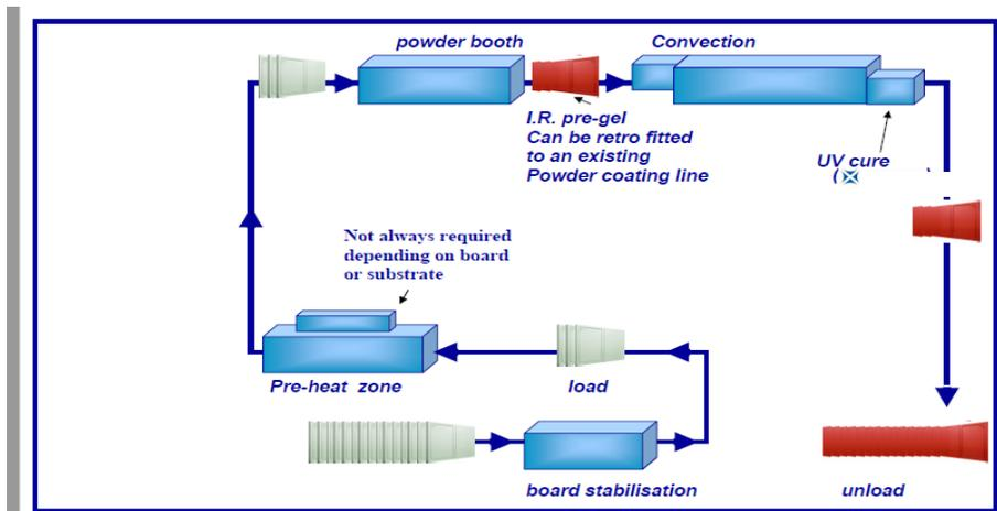
Figure 2: Powder Coating Layout
