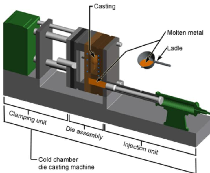
Figure: 1. Cold Chamber Die Casting Machine
