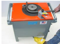
Figure 1: Current bending machine in South Africa
