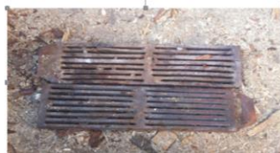
Figure 4 Fire grates of boilers at Nyanga pine
