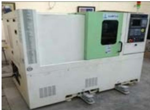
Figure 1. CNC Turning- LMW LL20TL3
