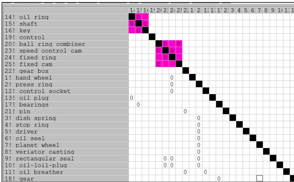
Figure 5: Components interdependencies within the case industry's product (gear) (clustered)
