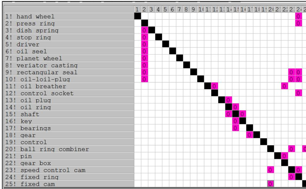
Figure 4: Components interdependencies within the case industry's product (gear) (un-clustered)
