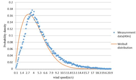
Figure 5. Abadeh probability density distribution of the wind speed at 40 m height
