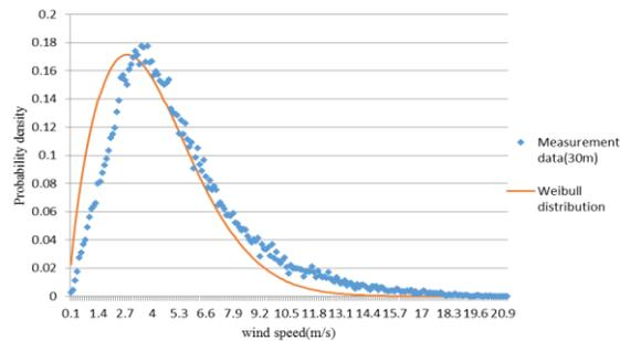
Figure 4. Abadeh probability density distribution of the wind speed at 30 m height
