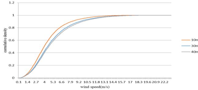
Figure 8. Cumulative distribution function at three height for Abadeh
