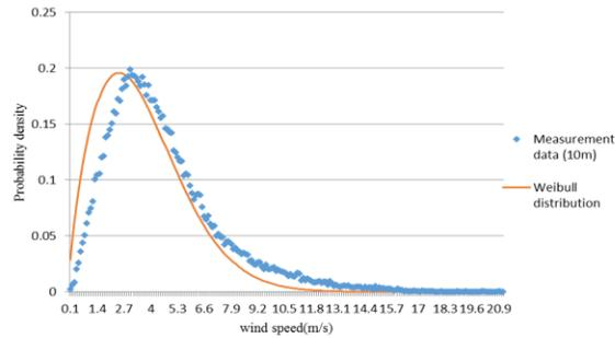
Figure 3. Abadeh probability density distribution of the wind speed at 10 m height
