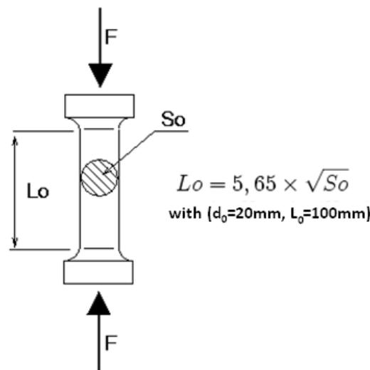
Fig. 1: Uniaxial compression test
