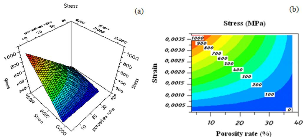
Fig. 3 Response-surface (a) and Iso-response (b) plot, showing the effect of porosity rate on the behaviour of Corundum
