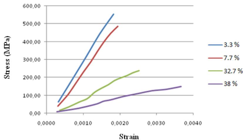
Fig. 2 Stress-strain curves of Corundum obtained at different rates of porosity
