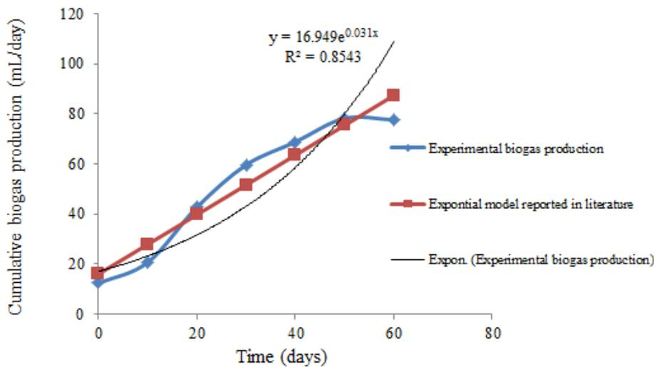
Figure 2. Comparison of the exponential kinetic model to cumulative experimental biogas data
