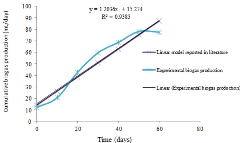
Figure 1. Comparison of the linear kinetic model to cumulative biogas experimental data
