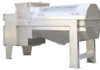
Figure 3. The peeling, pitting and extraction machine
