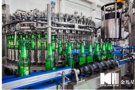
Figure 7. The bottling, encapsulation and labeling process in a Japanese company
