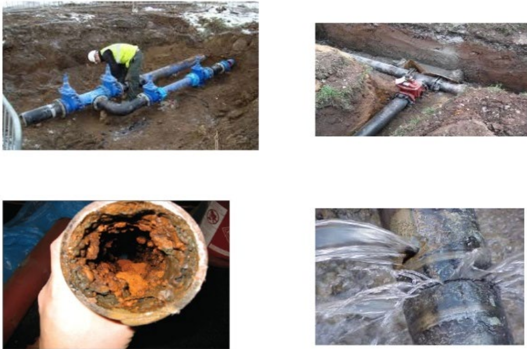
Figure 1. Pipe Deterioration Process
