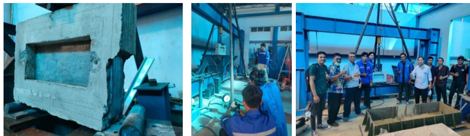
Figure 10. Compressive Strength Test of Concrete Puzzle Panel
