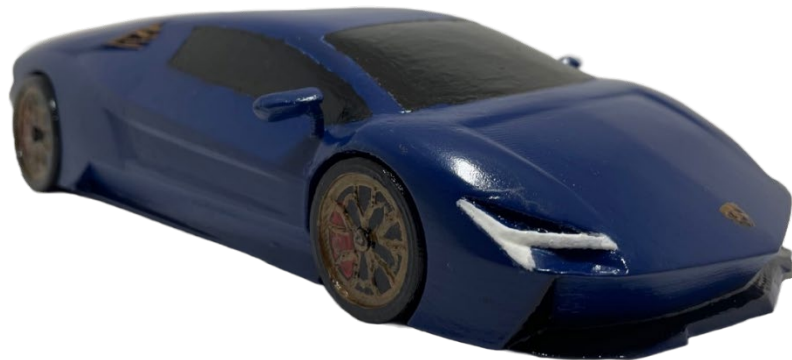
Figure 16. 3D physical prototype completed.
