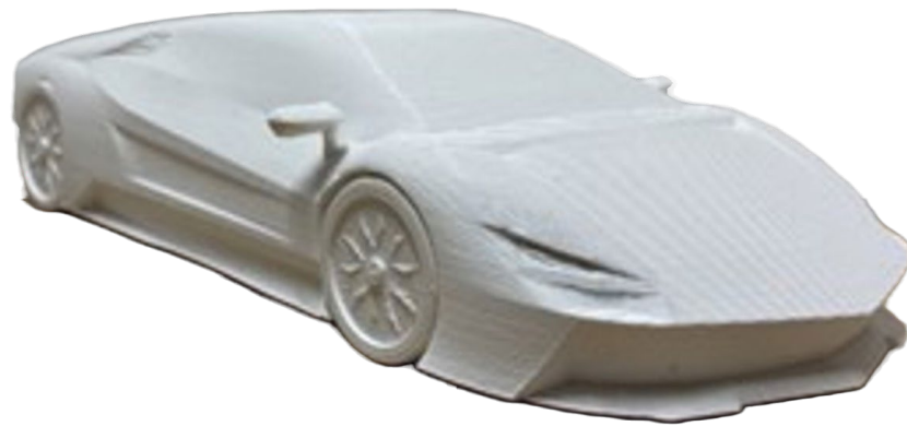
Figure 13. Views of the prototype post support removal.
