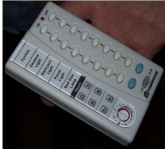
Figure 2. Remote control for lighting
