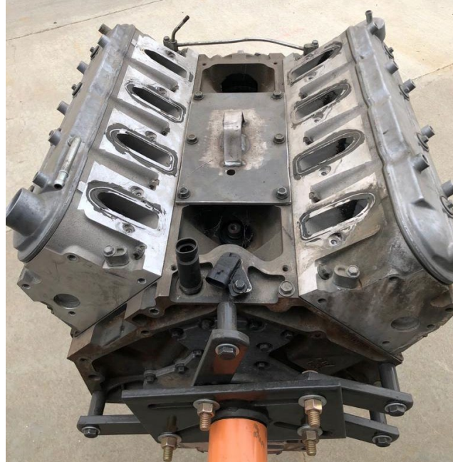
Figure 13. V8 Engine - Before Cleaning
