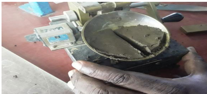
Figure 14. Depicts casagrande cup full of soil for liquid limit test
