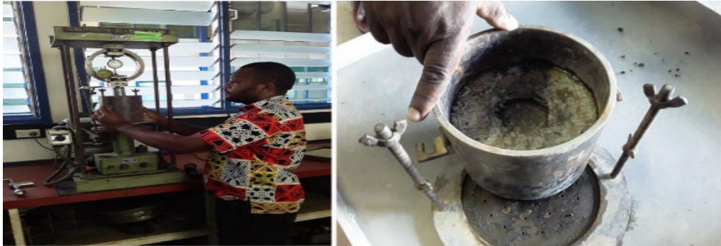
Figure 12. Ready for CBR penetration test (left), after penetration (33 mm depth)
