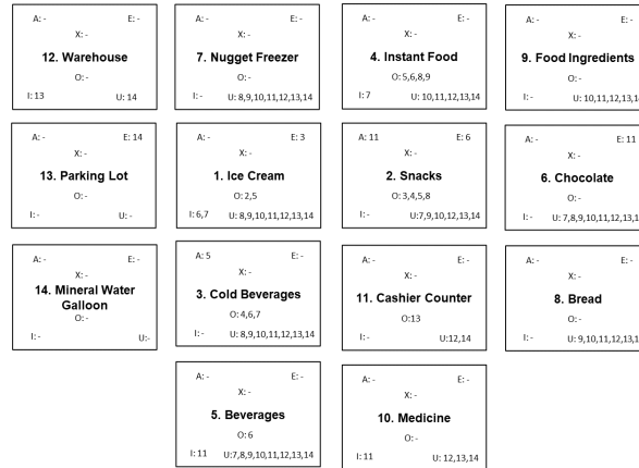
Figure 13. First floor ARD of Al Hikam Mart
