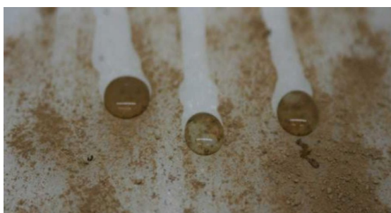
Figure 4. Picture depicting rolling down of water droplets carrying dust particles on a superhydrophobic surface (PV cells, 2017).
