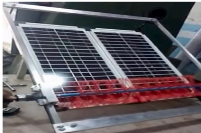
Figure 9. Brush cleaning system
