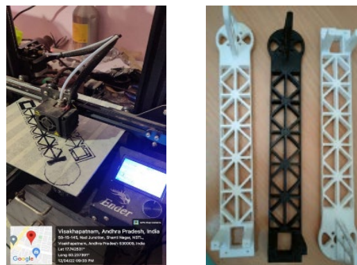
Figure 4. 3D Printing of components and 3D Printing arms
