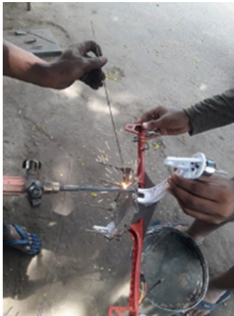
Figure 5. Fabrication of metal body for the drone
