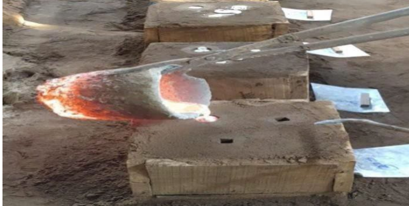
Figure 6. Pouring molten metal into mould.
