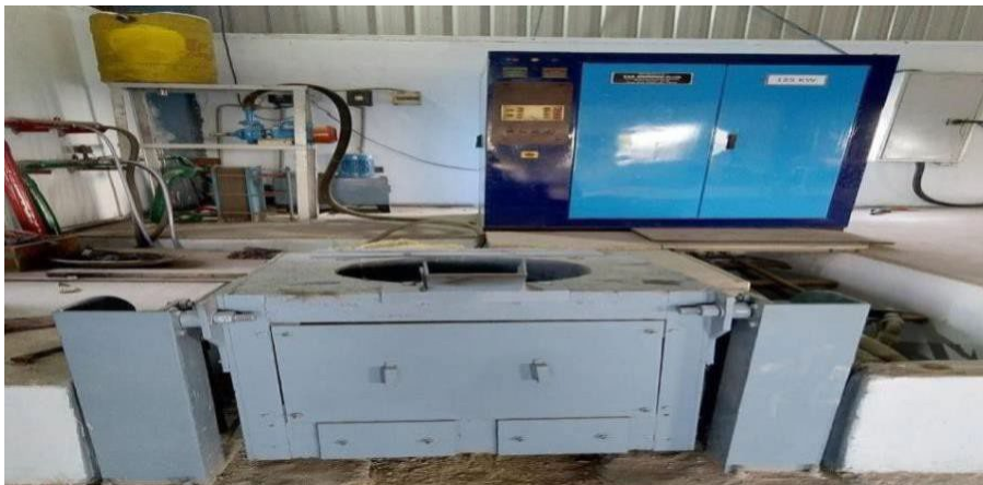
Figure 1. Induction furnace used to melt the aluminium scrap chips.
