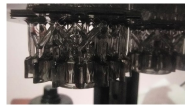
Figure 9: 3D printed gears on build plate
