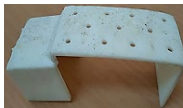
Figure 8: 3D printed motor Housing
