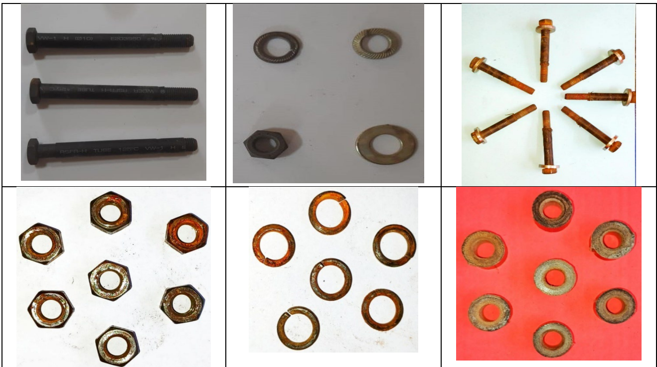
Figure 9. (a) As received MS Bolts with an insulating cover, (b) As received washers and nuts, (c) Corroded bolts after a service period of 2 years (d) Corroded nuts after a service period of 2 years, (e) Corroded spring washers after a service period of 2 years, (f) Corroded plain washers after a service period of 2 years
