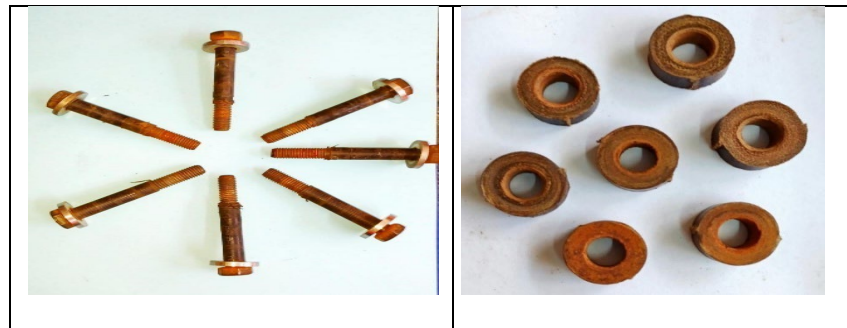
Figure 10. (a) Electrical insulating tube over MS Bolts after 2 years of service, (b) Bulged insulating sleeves after a service period of 2 years.
