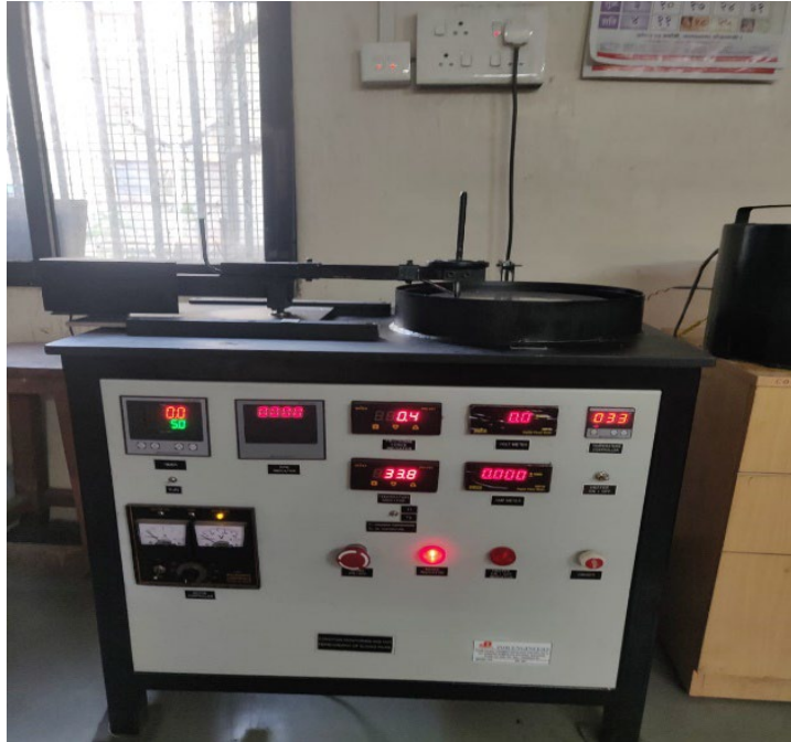
Figure 1. Pin on disc setup
