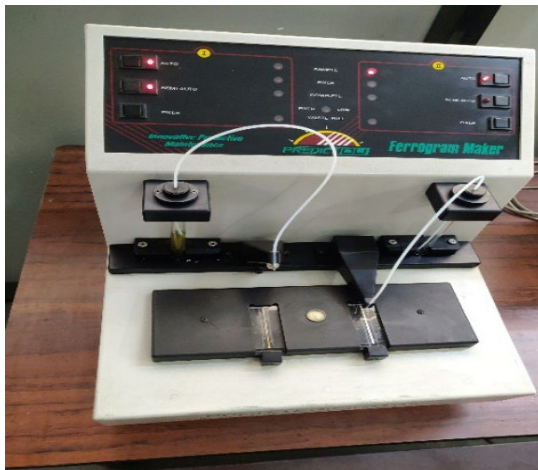
Figure 5. Dual Slide Ferrogram Maker
