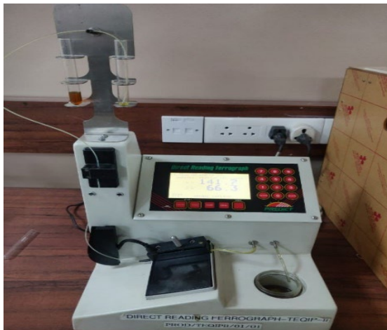
Figure 4. Direct Reading Ferrography
