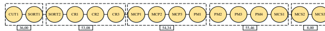
Figure 6. Division of Work Elements into Work Station Memo Square Glue Using the KW Method
