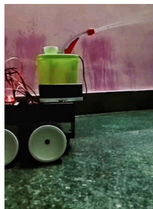
Figure 8. Spraying of sanitizing fluid by the robot
