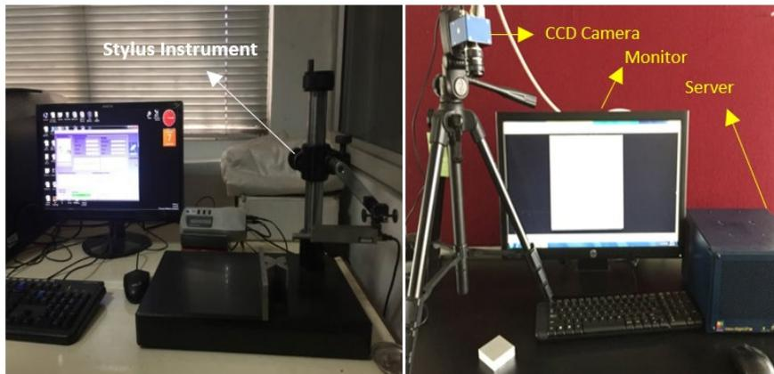
Figure 1 (a) Stylus instrument (b) Vision system and its component
