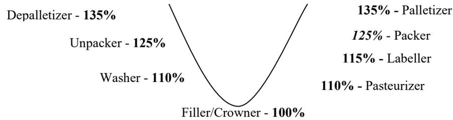
Figure 1. Line Layout (V-Curve)
