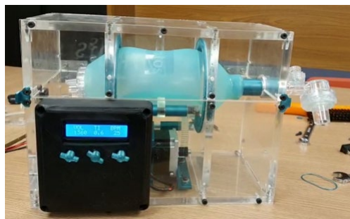
Figure 7: Ventilator built at the Technology Park of Sorocaba
