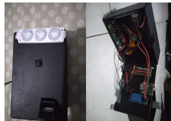
Figure 5. Implementation Door-locking System using Raspberry Pi Zero W (inside the box), a Webcam OV5467, AS608 – Optical Finger scanner, and Led for Illumination
