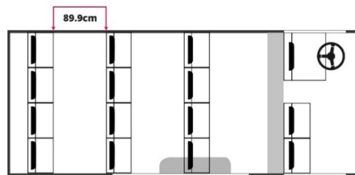
Figure 5 . Proposed design of the UV Express vans to satisfy the suggested anthropometric measurement
