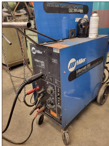
Figure 3. Millermatic 200 MIG Welder Machine in the lab
