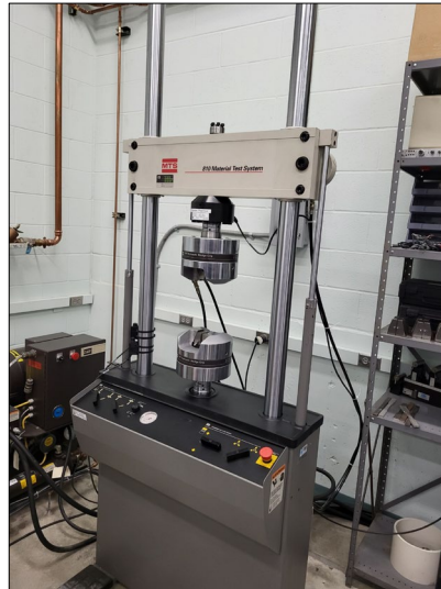
Figure 4. MTS Tensile Testing Machine in the lab
