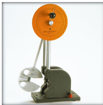
Figure 1. Impact Tester. Image source tercosweden.com (Terco, n.d.)
