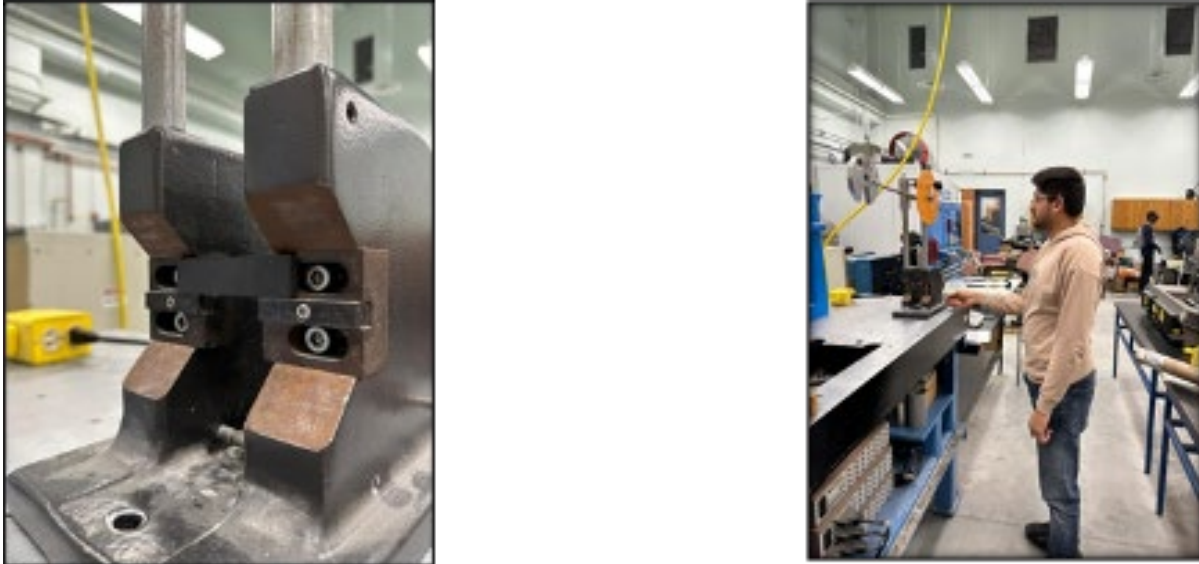
Figure 4. The figure on the left depicts the sample holder, while the figure on the right illustrates the direct energy measurements obtained from the impact tester, all of which are taken at the same height as the equipment.
