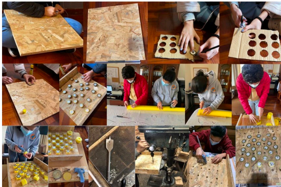
Figure 2. Piezoelectric disc placement process
