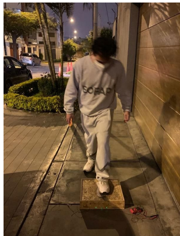
Figure 8. Piezoelectric tile working
