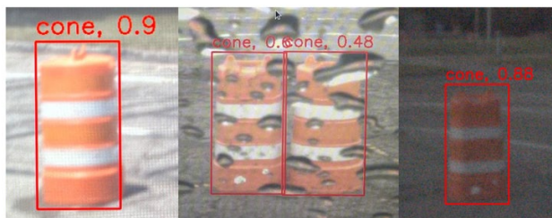
Figure 7. Sample cone detection in broad daylight, rainy weather, and after sunset
