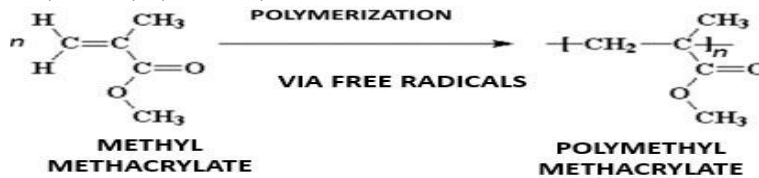
Figure 8. Equation for the polymerization of methyl methacrylate into 7-linden polymethacrylate.
