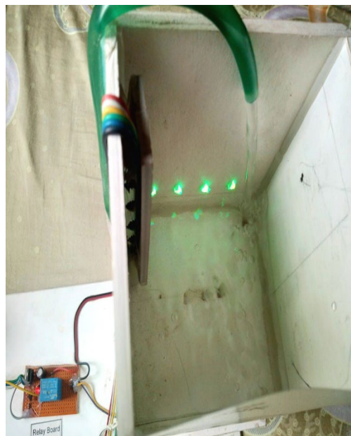
Figure 8. Motor ON and Water Flowing from Reserve Tank to Top Tank
