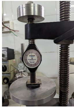
Figure 6. Conducting Shore D hardness Test
