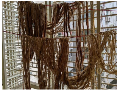
Figure 2. Drying fibers in sunlight
