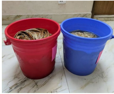
Figure 1. Chemical treatment process on the kenaf fiber
