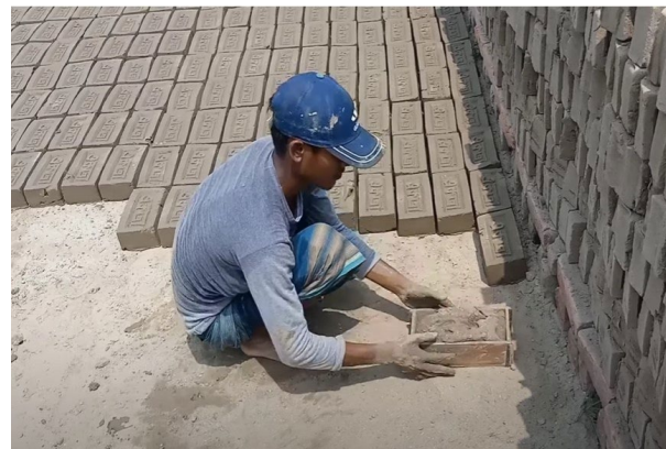
Figure 7(d) :Manual molding process.
