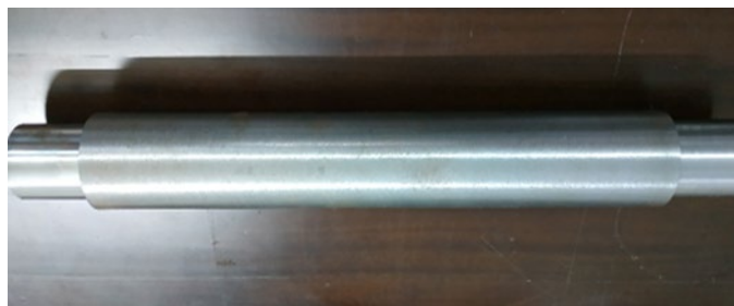
Figure 1. Experimental workpiece of hardened steel
