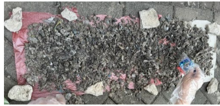
Figure 2. Waste Sludge Drying Process
