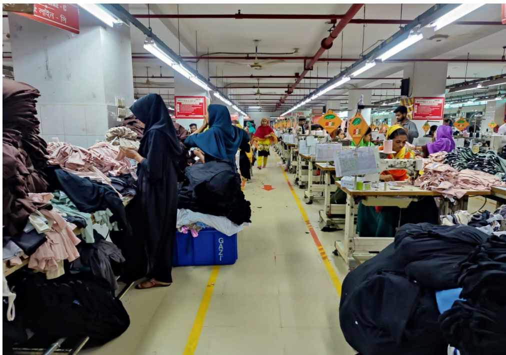
Figure 5. Progressive Bundle System (PBS)
