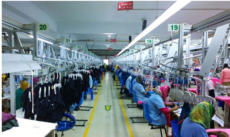
Figure 4. Unit Production System (UPS)
