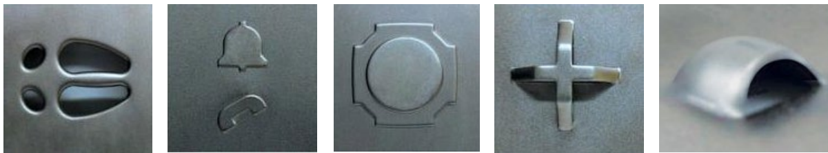
Figure 10. Examples of punching operation with special tools
