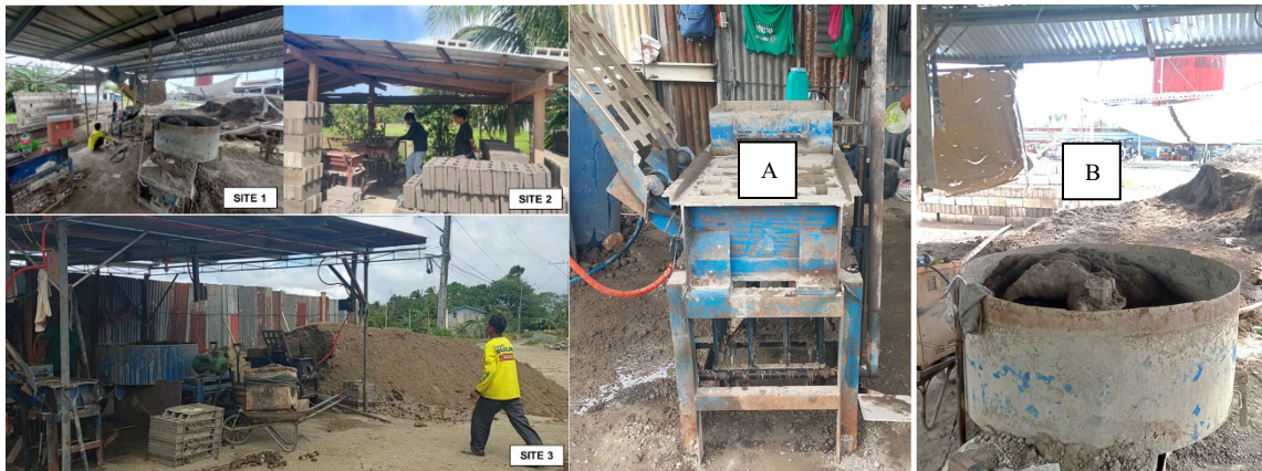
Figure 2. Hollowblock manufacturing sites at Lucena City; (a) stationary hollowblock making machine and (b) pan type cement mixer
